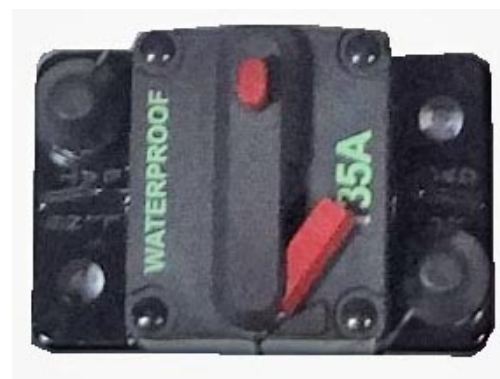
Switch pushed out
